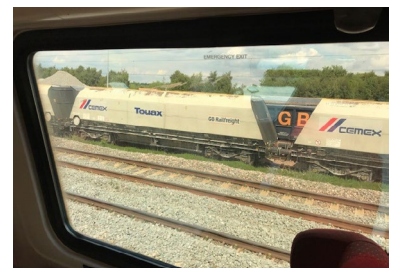
Coal cars converted into aggregate one
