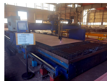
Plasma cutting of the first steel plate
