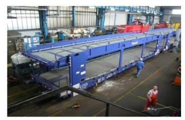
Manufacture of a car-carrier railcar
